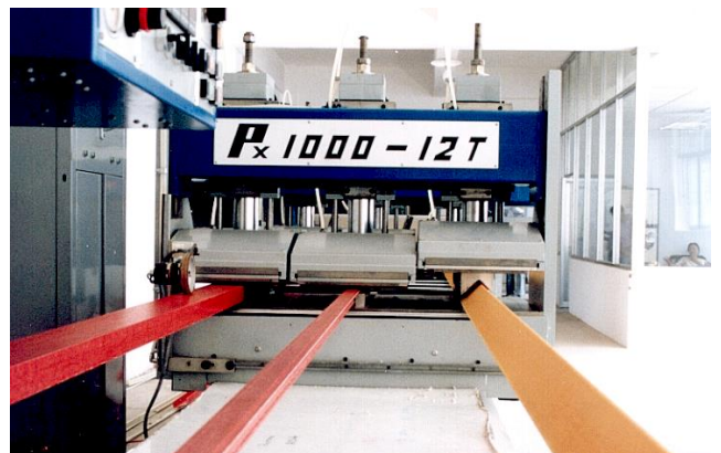
Pultrex 'first' with multiple clamp modules – allows maximum flexibility on larger machines
