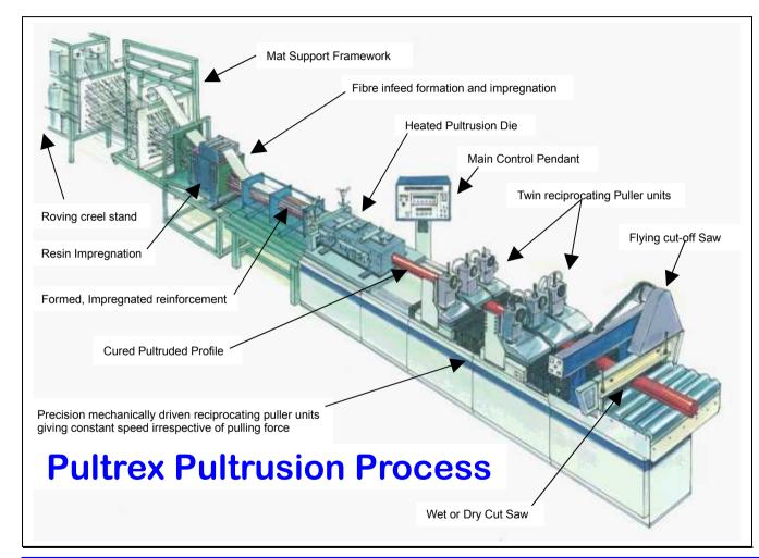
The Pultrusion process is a highly automated continuous fibre laminating process producing high fibre volume profiles with a constant cross section.
